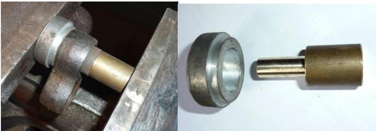
One tool effectively supports the link whilst allowing the rubber bush to emerge far enough to sit symmetrically in the link, the other tool is just a stepped drift that fits snugly into the rubber bush and has a shoulder that pushes the bush into position. The 'tools' are assembled in position and the bush simply pushed into position in a press (vice). Dead easy!
