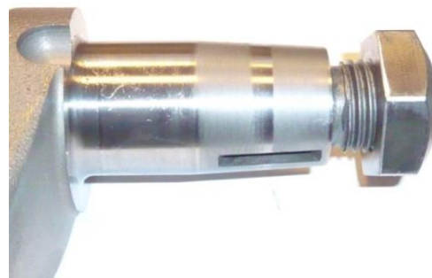
Matching crankshaft taper
