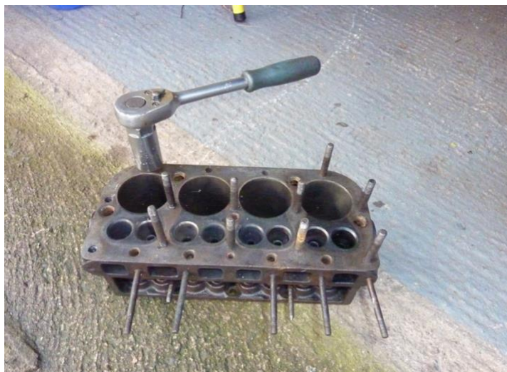
Using a 'roller cage' type stud extractor
