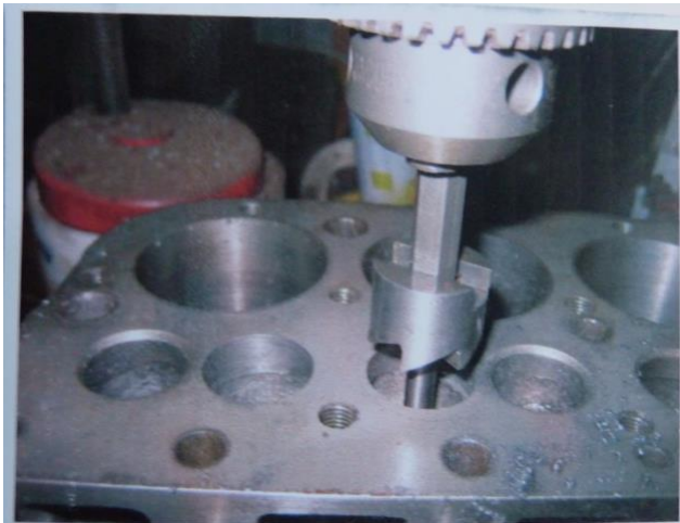
Boring for larger inlet valves
