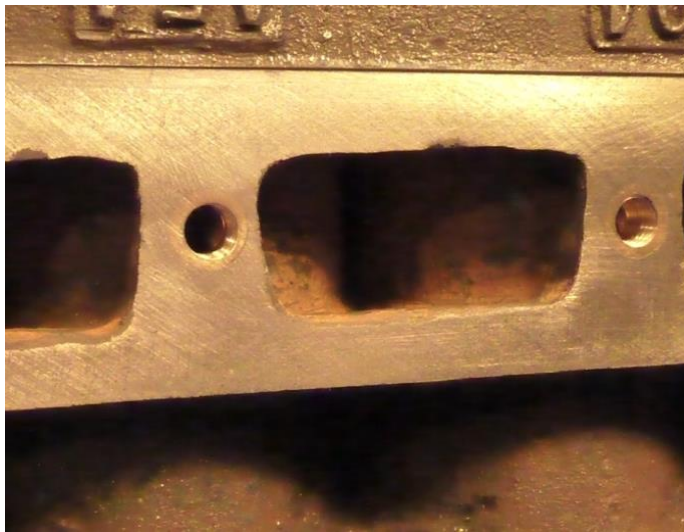
New bushes finished flush
