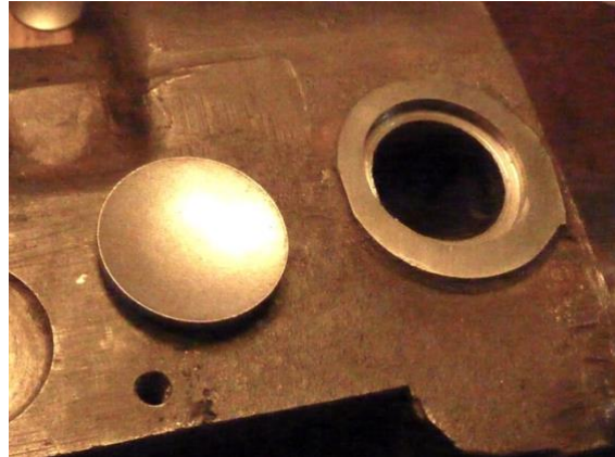
New core plug and clean seating
