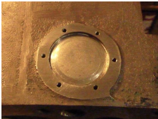
Plug fitted & 6BA holes tapped
