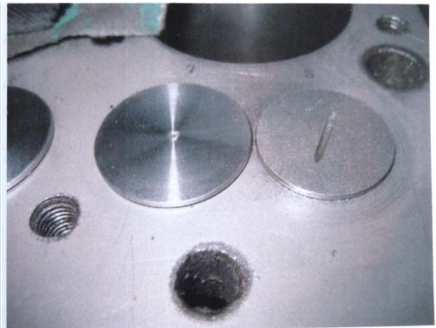
Large inlet valve in position
