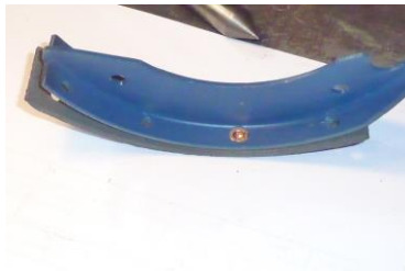
Rivet closed with drift
