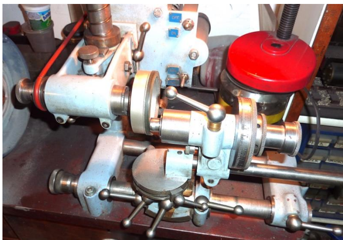
Refacing actuator plungers
