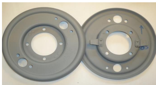
Backplates cleaned and etch primed
