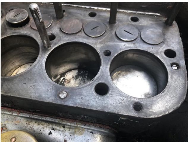
Two studs sheared off in block, at cylinder head level
