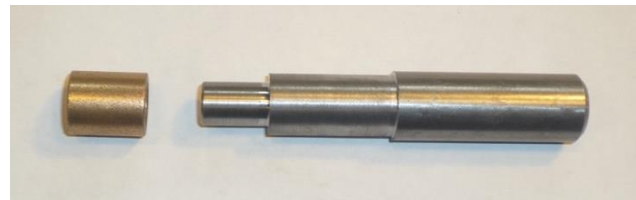
New 'Oilite' bush and bespoke drift
