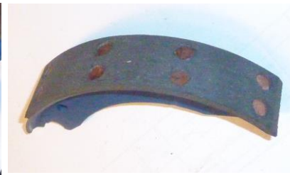
All rivets in position
