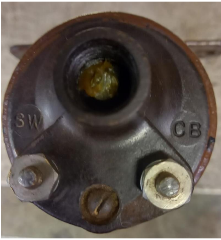
An early HT coil, showing the SW and CB connection Typical early Lucas, 80% of which were for -ve earth
