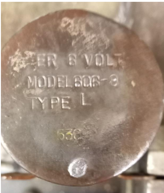
The underside of a 1936 A7 positive earth coil. This is from Eddie's Mk 1 Ruby, and probably 'Type L' indicates +ve earth The 536 refers to 5 th month of 1936.
