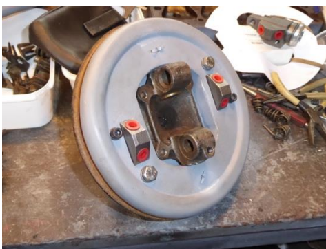
Fig 7 Inside view of assembled backplate
