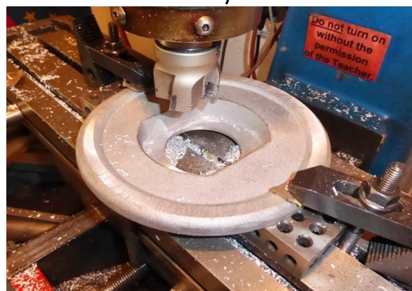
Fig 4 - Truing-up the inner face of the recess
