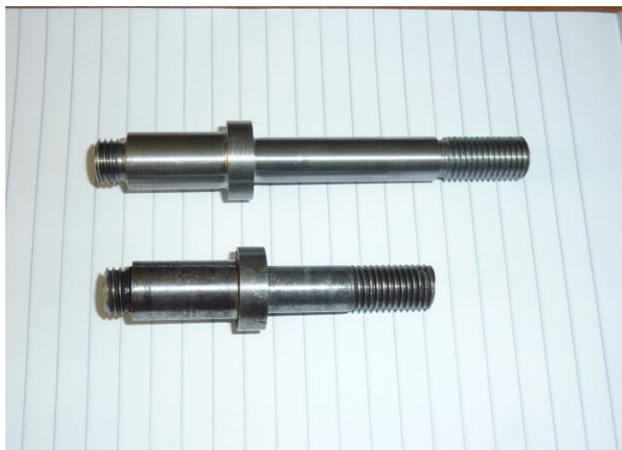
Fig 13 - Footbrake pivot pins (top as machined, bottom standard A7)
