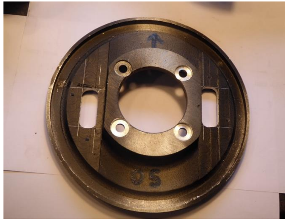
Fig 6 Cylinder positions marked-out
