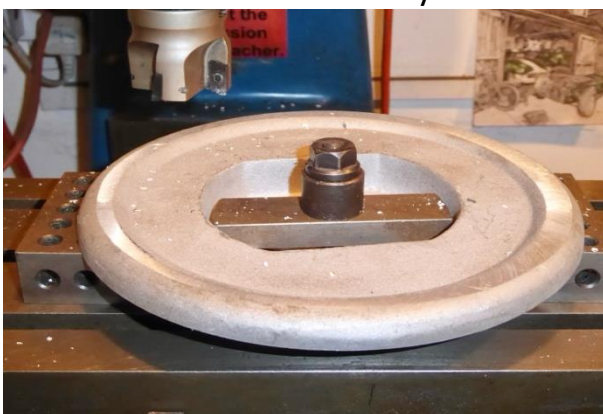
Fig 3 - A light cut on the inside of the rim
