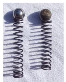
If this valve is worn, it can be the cause of abnormally low oil pressure. It needs to be routinely serviced every 25,000 miles, or when the engine is rebuilt. The valve protects the oil pump by preventing the oil pressure getting too high. This occurs when the engine is cold and the oil is more viscous. The valve is located on the left side of the sump, but is obscured by the chassis rail.
