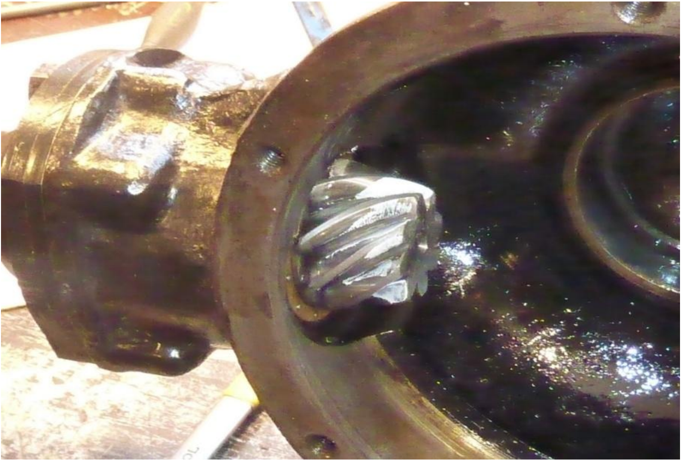
Pinion markings at first assembly
