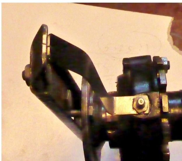
Index marks used to check 1/16" of backlash at 7" radius
