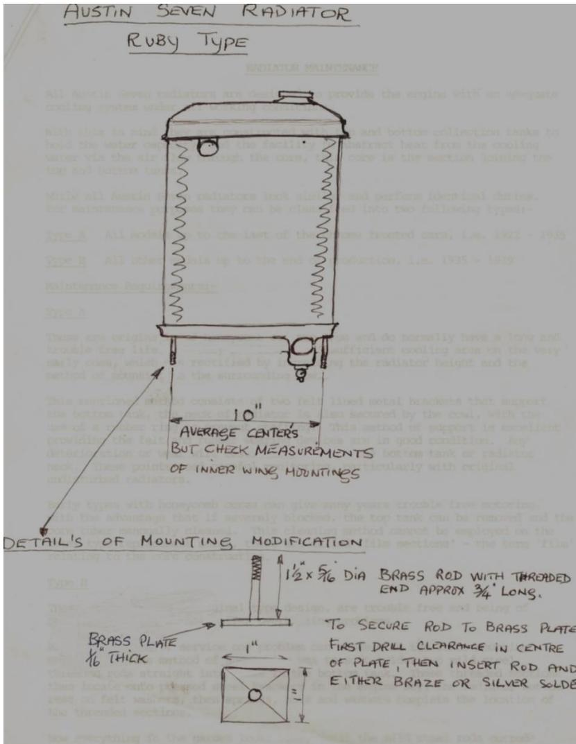
3. Carefully mark out the measurements of the engine bay support brackets onto the bottom tank, thus ensuring that when the brass plates are soldered into position, they correspond with their counter parts in the engine bay.
