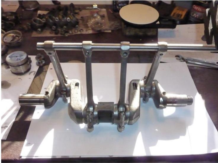
length of 0.500" diameter ground Silver Steel through all four little ends with the rods firmly attached to the crankshaft. For new members and those with an imperfect memory, we have a similar photo here on the left.
