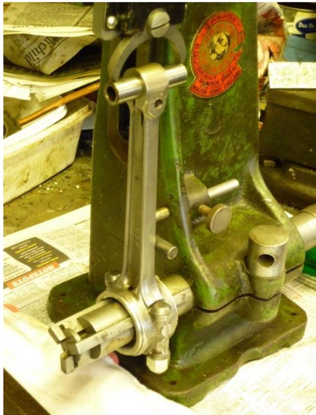
Eddie assures me that slightly bent rods can be straightened satisfactorily. Very slight adjustments by cold twisting or bending are considered permissible. Usefully, the Dorset A7 Club website Technical Pages show how rods can be straightened using a vice as a press.
